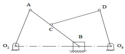
(h) Design a four bar linkage in which two successive clockwise angular displacements of 20° and 30° of the crank produce respectively, two successive angular displacements 10° and 15° of the follower.
