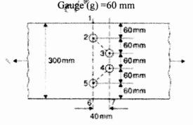
b) Determine the block shear strength of the welded tension member shown below .grade of steel is Fe 410.
