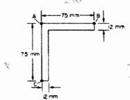
(b) The bending moment acting on the curved beam with a rectangular cross-section is M = 8 KN-m. Calculate the bending stress at point B.
