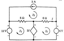
Determine the currents in the various branches of the circuit shown below by nodal (b) analysis.
